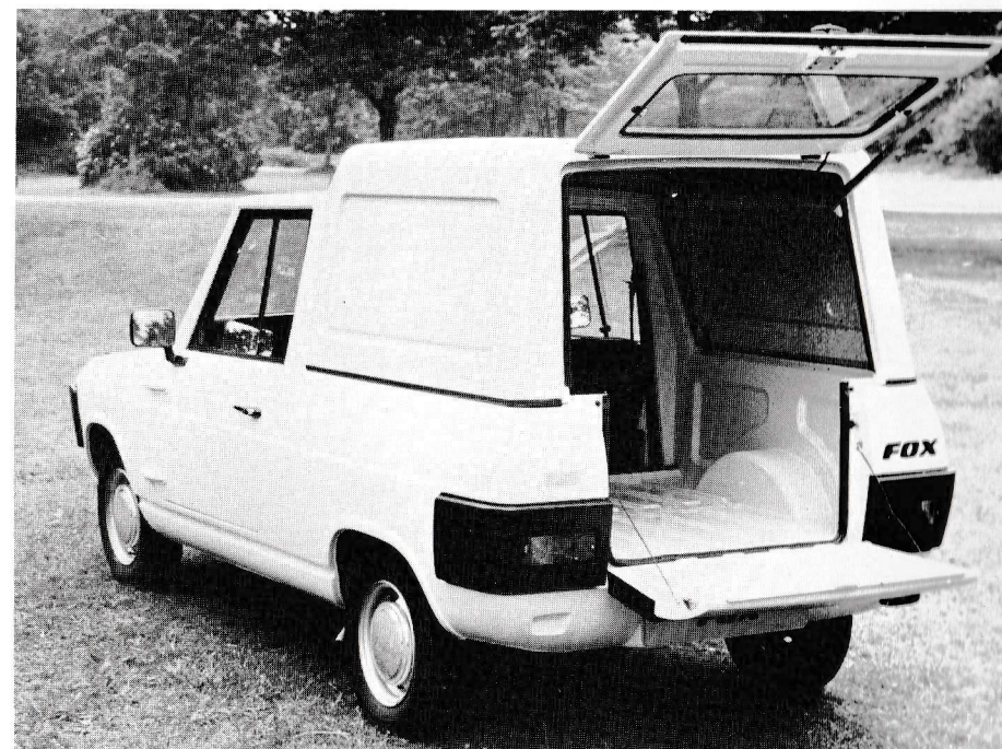
The 50 cu. ft. (1.4 cu. m.) Fox Hardtop has a top hinged rear door and heated rear window.
