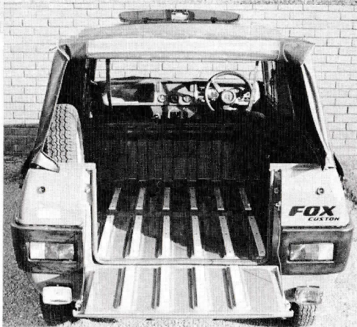
The Fox Utility features a black PVC tilt on removable steel hoops with a roll-up rear window. (Vehicle shown is fitted with custom pack and load space bulkhead options).
