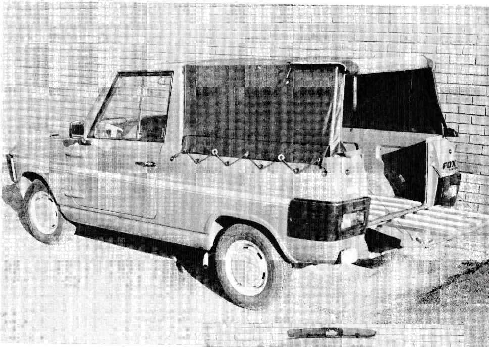
The Fox Utility features a black PVC tilt on removable steel hoops with a roll-up rear window. (Vehicle shown is fitted with custom pack and load space bulkhead options).
